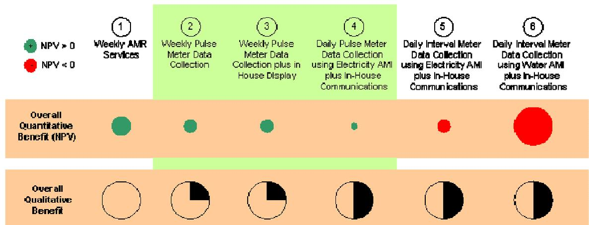
Interval metering is comparatively more expensive than pulse metering as the meter is required to constantly monitor the water flows through the meter and record this volume at the expiration of the metering interval.
