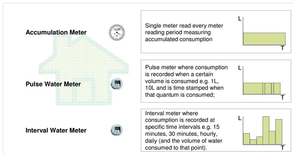
The past decade has seen an evolution of conceptual design of advanced or smart metering and its terminology. Driven by electricity investment, metering has evolved from accumulation meters to interval meters with simple communications, to advanced or smart metering with an increased range of metering functionality. This increase in electricity meter functionality and complexity has started to be mirrored in the water industry.
